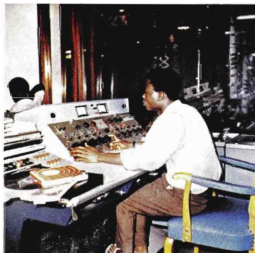
FIG. 6 BC-7A Console uses stereo channel for standby.
