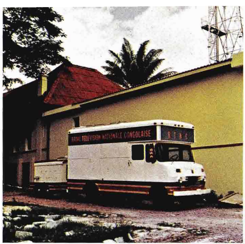
FIG. 2 Mobile unit, decorated in the national colors, transports cameras and tape recorder equipment to remote locations for telecasts of sports.
