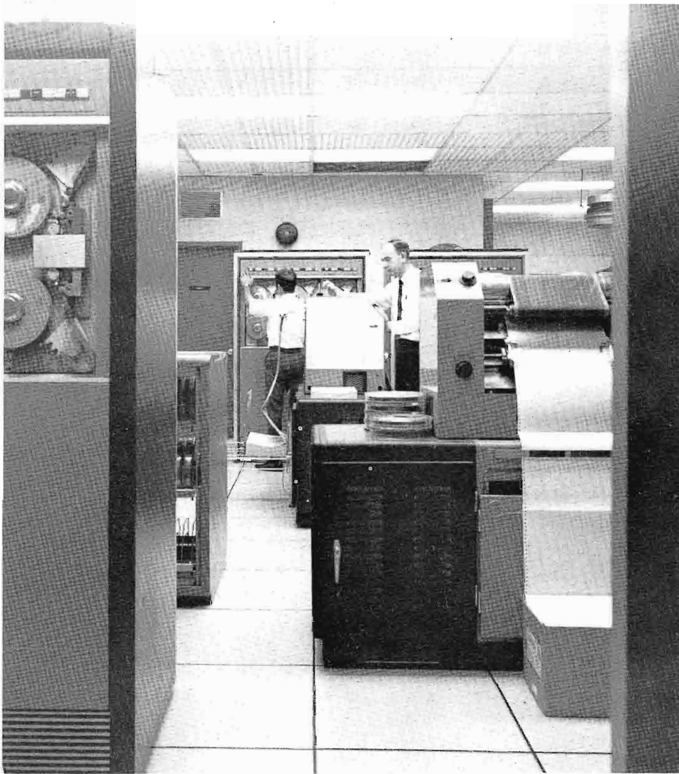
FIG. 2 Two RCA 301 Computer Systems give answers to complex requirements in minutes that would otherwise take months. This highly sophisticated computer system writes at 1200 lines per minute to maintain parts inventories.
