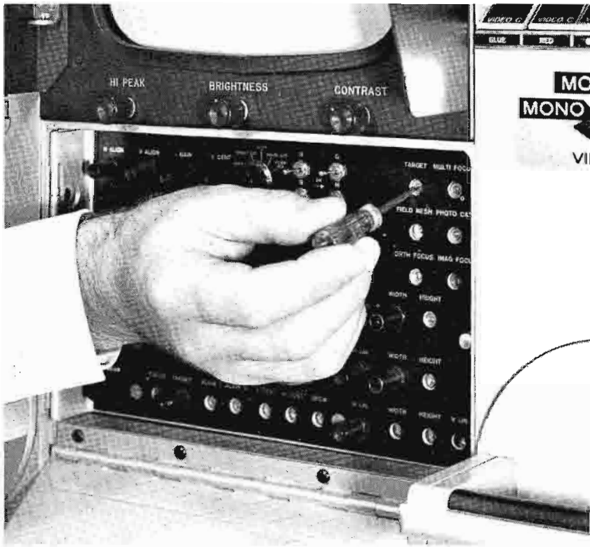
FIG. 2 Adjustment of target voltage.
