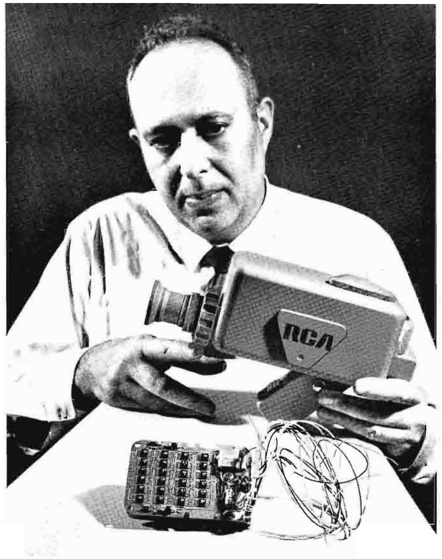
FIG. 3 The use of integrated circuits made it possible to produce a 4½ pound miniaturized TV camera. Hundreds of IC's are contained in the black squares on this circuit board from the Apollo camera.
